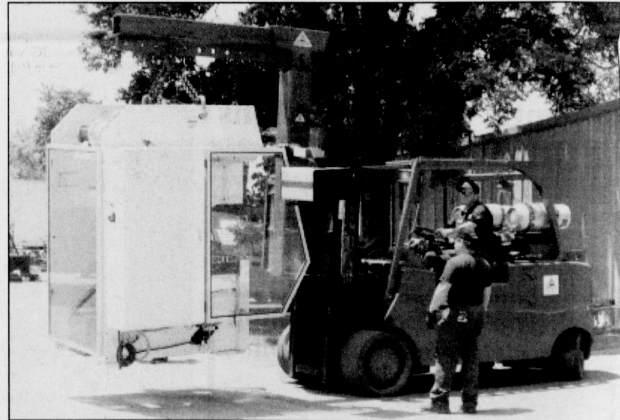
NEW PRESS BRAKES are unloaded at Contico by a forklift company from Dallas/Ft. Worth. The five new machines were purchased in Connecticut and are used to bend sheet metal to make tool boxes. The new, state-of-the-art equipment will eliminate 14 old, outdated, World War II-era machines. The press brake above is the smallest of the five, weighing about 15,000 lbs.
