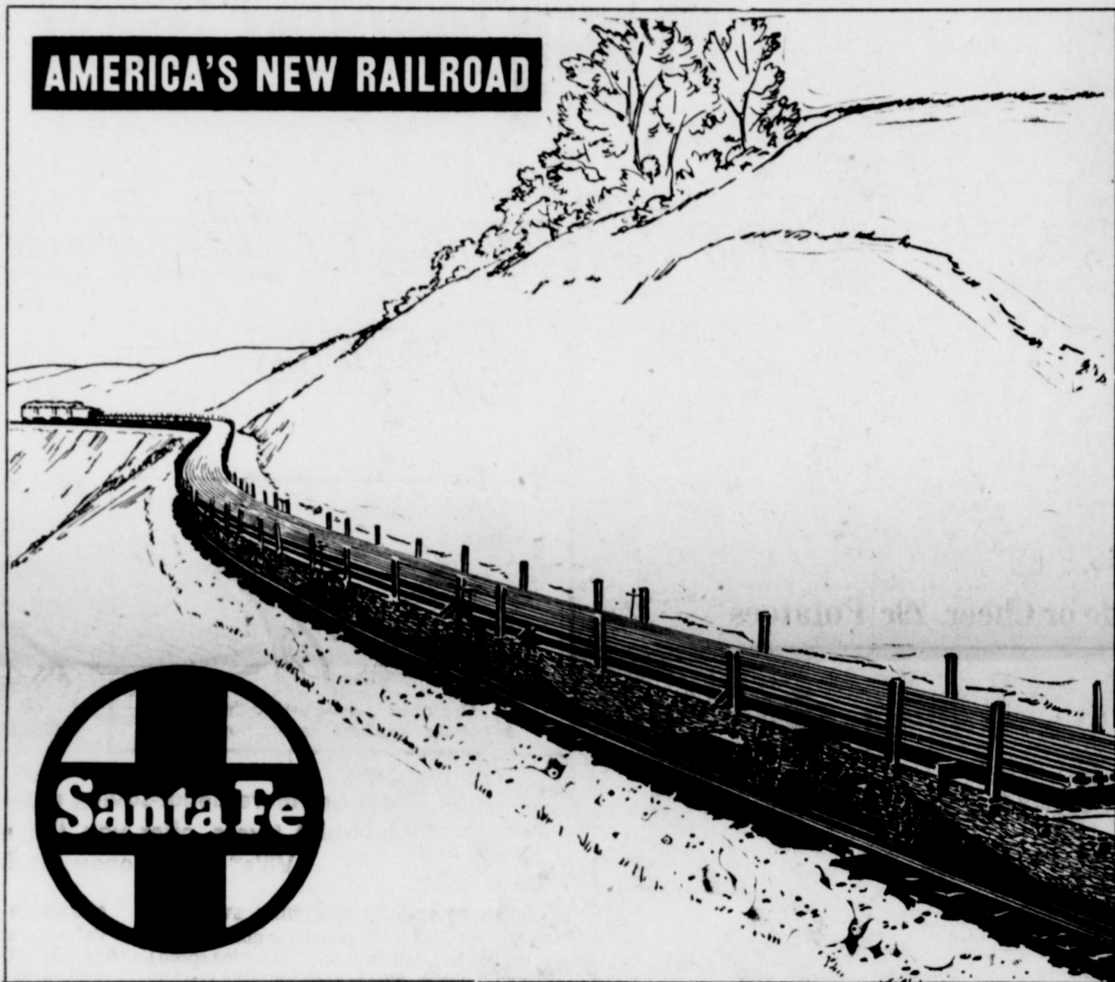
Quarter-mile lengths of welded steel rail curve around a foothill like wire cable.
