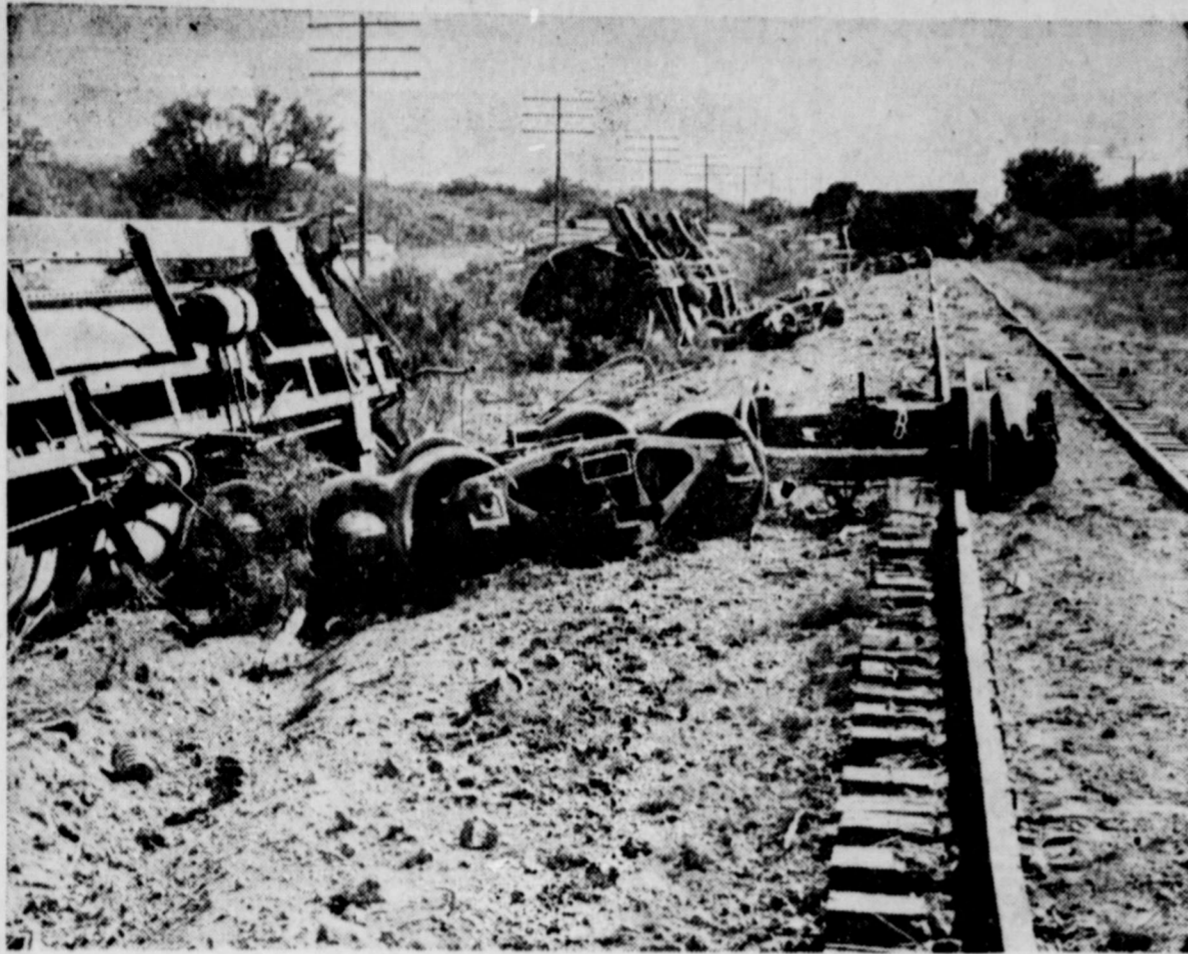
ON THE WRONG TRACK —Scattered over a wide area are 11 tank cars and the caboose of a Santa Fe train which jumped the track about 2:45 p.m. Sunday, this side the county line south of Tennyson. The cars were torn loose from their axles and wheels when the accident occurred. Santa Fe official blamed twisted rails caused by excessive heat for the accident. The train was headed north, going from San Angelo to Sweetwater. —Photo Courtesy Standard-Times
