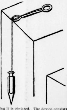
ing it is obviated. The device consists of a holder of wire, about which the surplus cord is wound, with looplike coils on each end.
