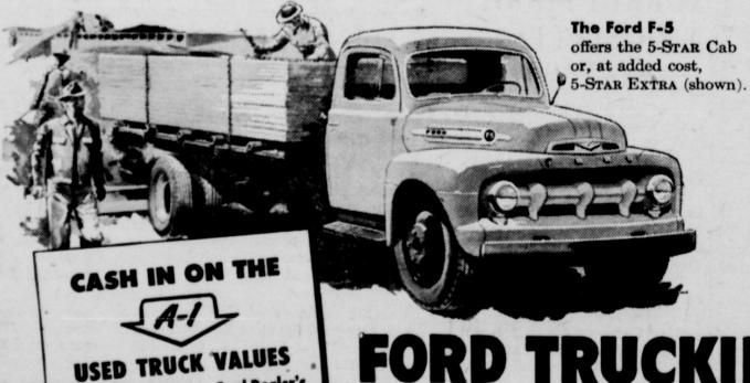
Only 11/2-ton truck offering choice of high torque 106-h.p. V-8 or all-new LOW-FRICTION 101-h.p. Cost Clipper Six! Saves up to one gallon in seven!
