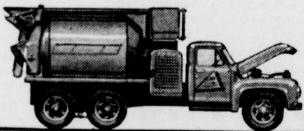
NOW 1 TON MORE GVW —Ford T-800 tandem now has 42,000 lbs. GVW. 170-h.p. Short Stroke V-8. 11,000-lb. front axle available. New capacities also apply to Cab Forward models.
