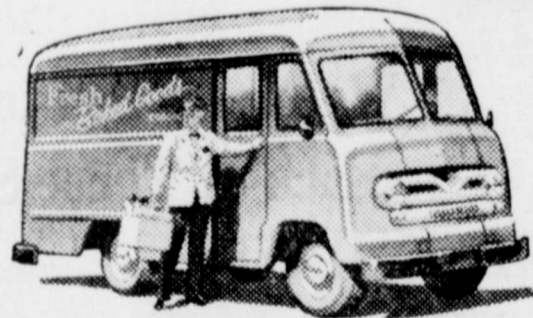
P-350 Parcel Delivery handles bodies up to 450 cu. ft. capacity. Fordomatic Drive, power brakes available.
