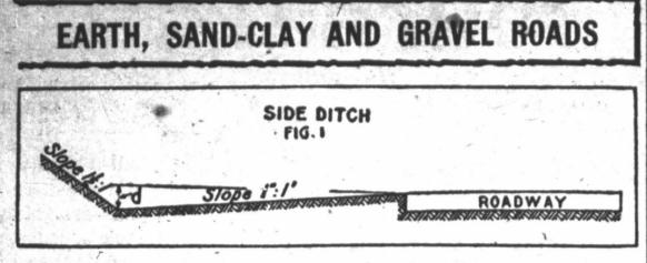
the very first consideration in connection with the location and design of any road. This statement requires no explanation, because the action of water in changing clay into mud and in causing all kinds of soils, except sand, to give way when a load is applied, is familiar to every person living in a humid climate. The following summary supplies a few suggestions as to how water may best be removed from a road bed:
