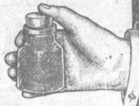
In this little bottle are 30,000 steel balls, every one of which has been tested and found to vary not one ten-thousandth of an inch. Fifteen balls are used in the bearings of every typebar. This attention to minute detail means efficiency for the finished product.
