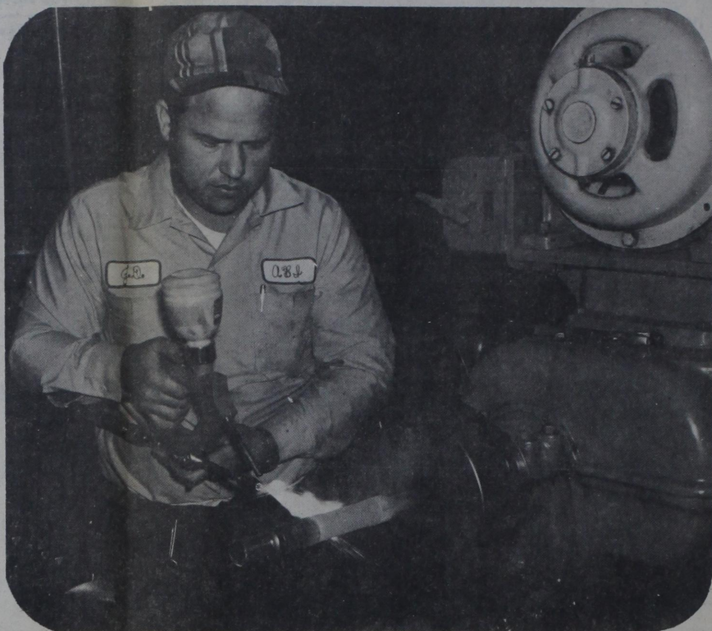
ROTOTEC GUN AT WORK —Shop Foreman J. D. Parker uses the new RoToTec Gun to rebuild a steel shaft with hard brass. As the shaft turns on the lathe, the RoToTec Gun applies a fine brass dust with a blue gas flame for a smooth, even buildup.
