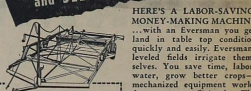
MODEL 25—Width 12'10", length 32', cutting blade length 9'3", depth 22", requiring 38 H.P. (drawbar).
