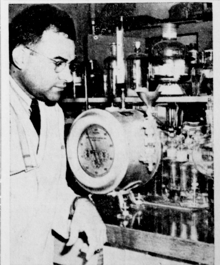
STINKOMETER—Dr. Lionel Farber of the University of California stands beside gadget which determines whether fish is fresh or a bit on the odor side. No unsavory sniffing is required because Stinkometer tests freshness chemically.
