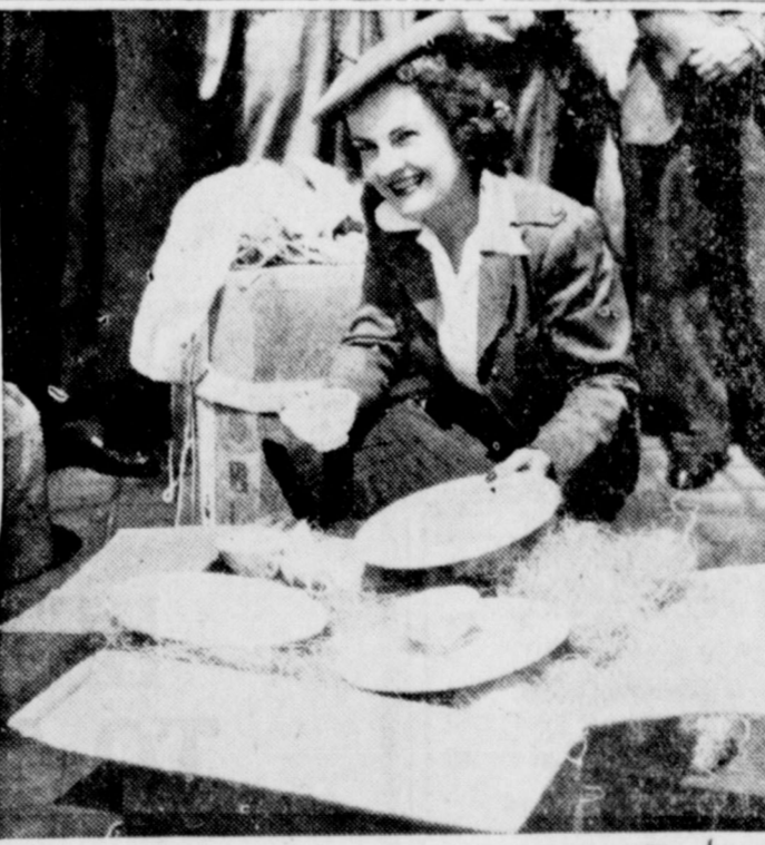
AIRBORNE CHINA—Chief Hostess, PCA, Katherine Hartman, opens box of dinner ware dropped by parachute during demonstration in Washington. Dishes were packed for ordinary air express shipment and came through drop unbroken. Demonstration proves towns not on air route can be serviced.
