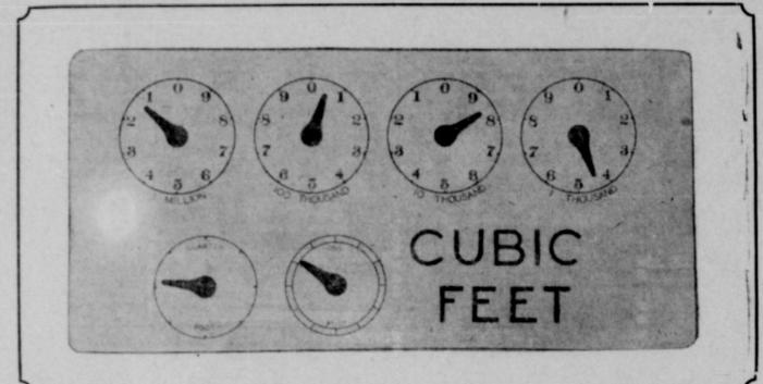
There is nothing mysterious about the reading of a gas meter. The ability to read a meter will acquaint patrons with the rate with which gas is being consumed on their premises. A meter also is valuable in detecting leaks.
