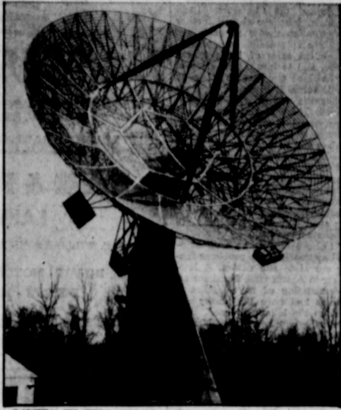
LISTEN TO THE STARS —That's what Harvard's astronomers plan to do with this 60-foot diameter radio-telescope at Agassiz Station, Mass. Largest in the United States, the "ear" is designed to pick up electrical impulses from stars as far as one hundred million light years into space. (A light year is equivalent to the distance traveled by a beam of light in one year at the rate of 186,000 miles per second.)
