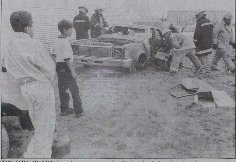
THE JAWS OF LIFE is an important piece of equipment for Dimmitt's Volunteer Fire Dept. Here, firefighters demonstrate the use of the tool to
