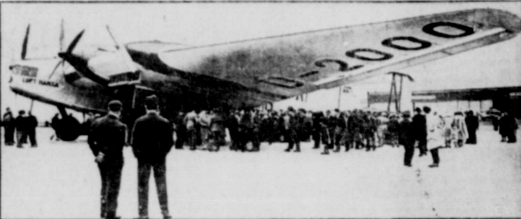
Germany's latest bid for leadership in airplane design is the giant machine shown here—the largest land plane in the world. It is a Luftwaffe Junkers, recently completed and sent on a test flight to Croydon Airport, England, where you see her here. The G-38, as it is called, is powered by four motors. Quarters for 14 passengers and a crew of six occupy part of the leading edge of the extremely thick wing where it meets the fuselage.
