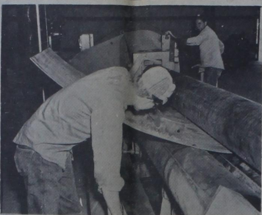
DON SAIN ROLLS CARBON-STEEL SHEET While Danny Christian checks curvature angle
