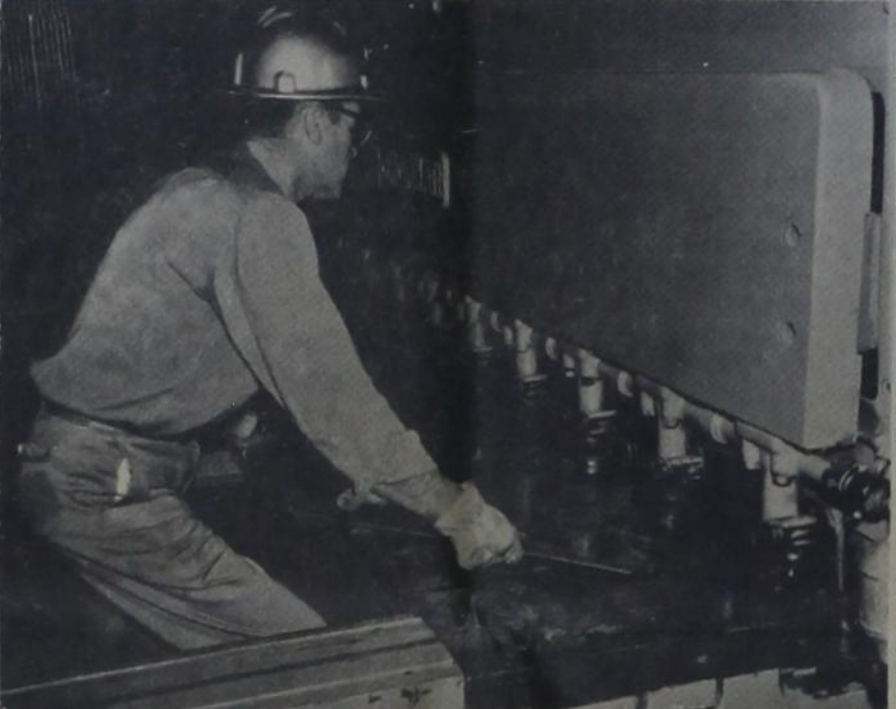
AL LYTLE OPERATES SQUARE SHEARER ... Cutting .16-gauge stainless cone section
