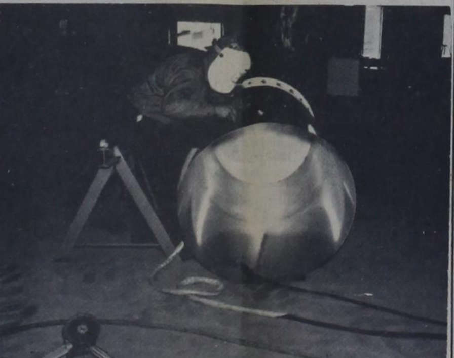
DEAN CANNON, WITH HELI-ARC WELDING UNIT ... On a stainless steel germ tank
