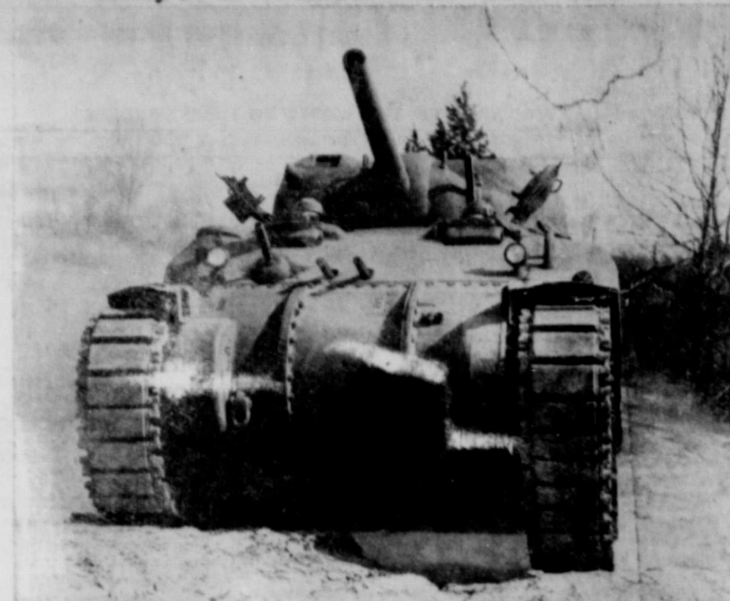
Thundering over a rough at... the Army's new rivetless medium tank complete with 75 mm. gun and a battery of machine guns.
