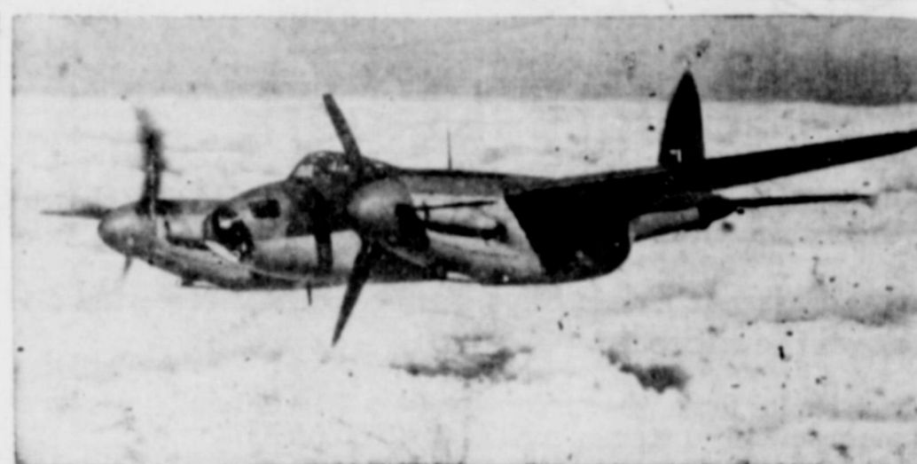
CAN'T SLAP DOWN THIS MOSQUITO—Cleverly designed new British Mosquito twin-engine reconnaissance bomber, demonstrates its ability to keep on flying even when one motor has been knocked out. One of the De Havilland three-bladed hydro-matic type propellers remains stationary as the ship skims the clouds. Offensive armament carries a powerful sting, with four 20-mm. cannon and four .303 machine guns to get under the enemy's skin.
