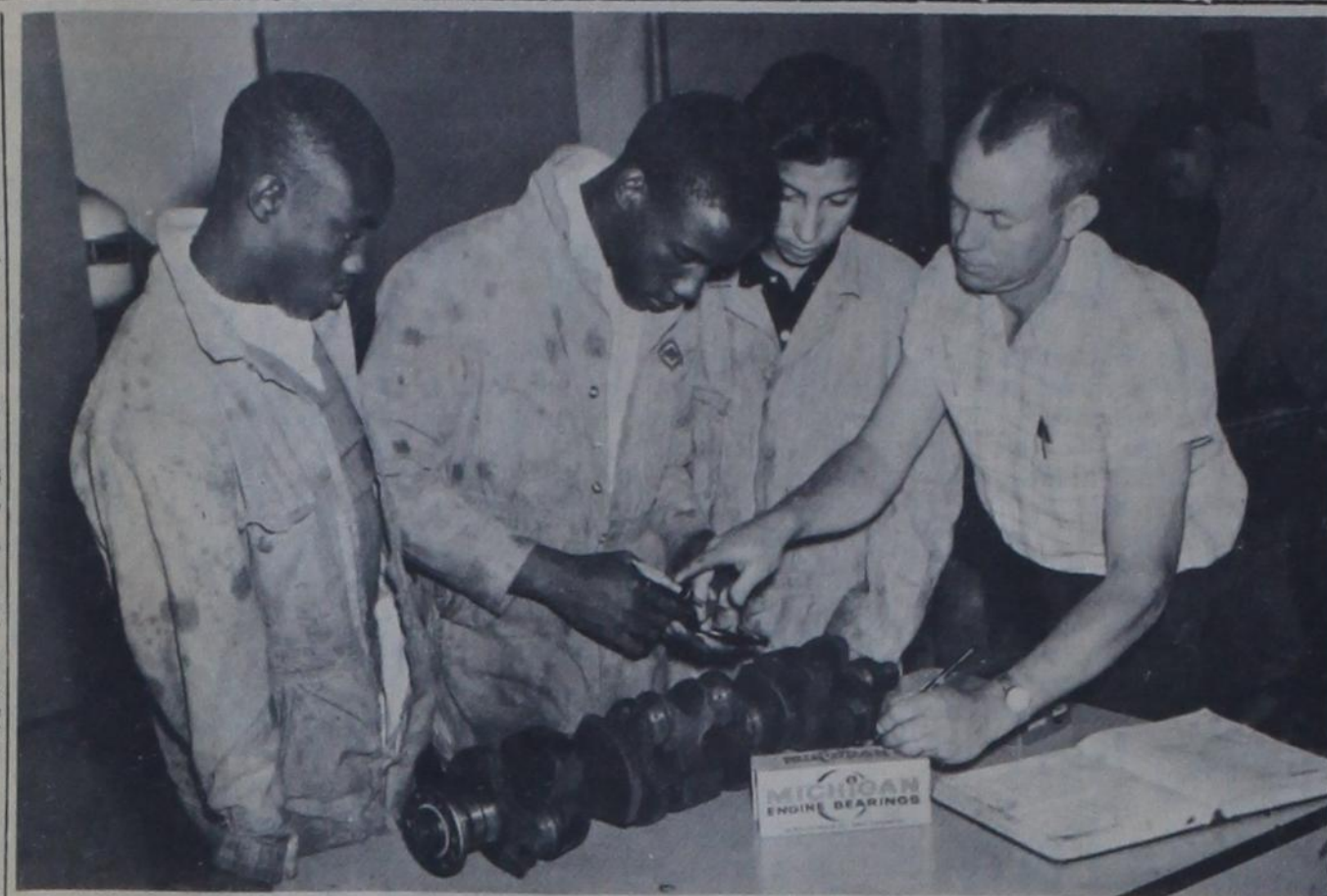
LEARNING TO 'MIKE' a crankshaft in Dimmitt High School's occupational training program are (from left) Roy Thomas, 17, Nelson Chavers, 15, and Ruben Herrera, 17. Jim Dowty (right), instructor of the course, shows the boys how to "read" a micrometer. The training program, conducted under Title I of the National Secondary Education Act, includes two-hour daily classes in such vocational trades as power mechanics, metal working and general repair.
