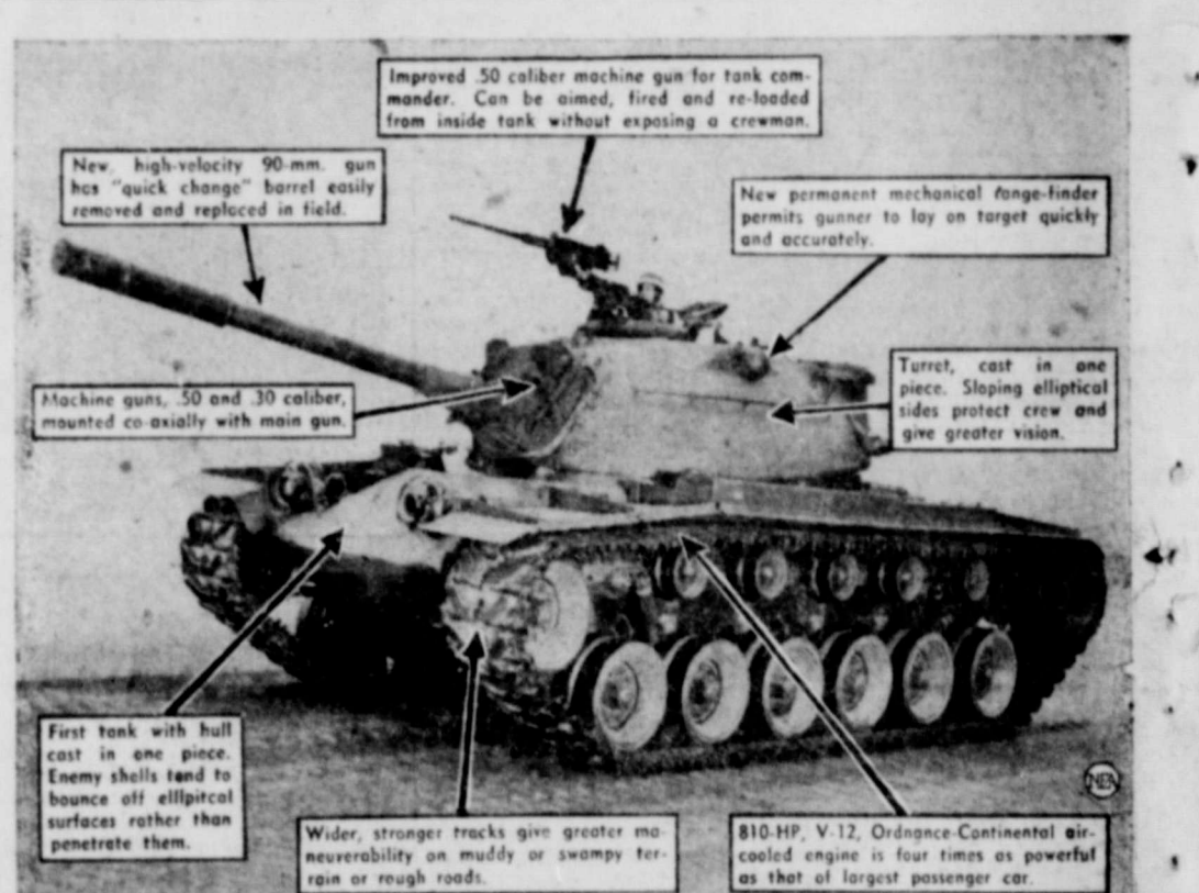
Here's the first picture of the Army's newest and most advanced medium tank—the long-secret Patton 48. It has just been officially unveiled and officially christened by Mrs. George S. Patton, Jr., at the Chrysler Delaware tank plant at Newark, Del. Most striking characteristics of the 45- to-50-ton monster are its low silhouette and new design, featuring elliptical-shaped hull and turret.
