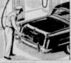
CENTER-FILL FUELING - prevents hose marks, and makes "filling up" easier from either side of the gasoline pump.
