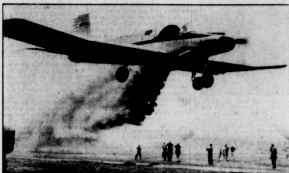
AERIAL FARMHAND —Swooping low to show off its crop-dusting ability, the "Fletcher Utility" goes through its paces at Rosenond, Calif. It is said by its manufacturers to be the first plane specifically designed for farm work to be put into volume production. Of all-metal construction, and with a 42-foot wingspan, the aerial workhorse is designed to pick up a 1250-pound load from an 870-foot, unimproved flight strip.
