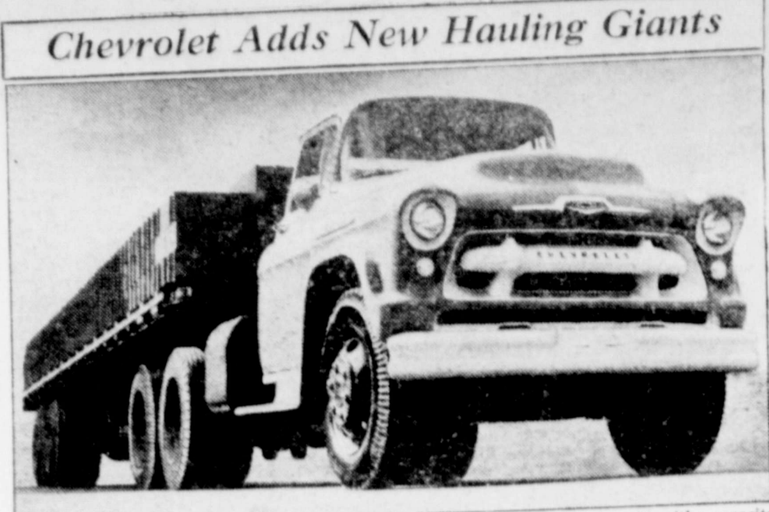
Chevrolet introduces for 1956 the heaviest commercial vehicles the company has ever manufactured, with 48 new models in the 2 1/2-ton class. For the first time, the company is offering optional tandem axle equipment. The tandems provide a number of the new units with a capacity nearly double that of any previous Chevrolet truck. Pictured here is a tandem-equipped 2 1/2-ton tractor with 17 1/2-inch wheelbase pulling a flat bed trailer loaded with concrete blocks.
