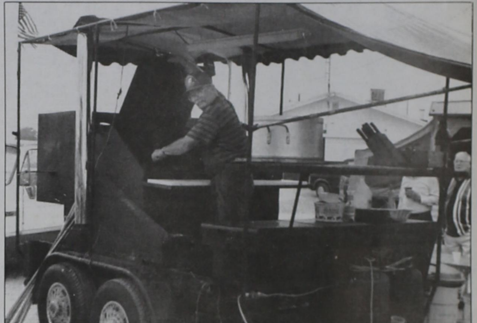
SERIOUS COOKING MACHINE—Don Hardy of Midlothian, a 1954 graduate of Dimmitt High School, checks the barbecue in his custom-built, tandem-axle cooker during the cook-off at the Castro Memorial VFW Post Saturday. The large cooking chamber has a motor-driven rotisserie and its racks can hold up to 500 lbs. of meat, although Hardy cooked "only" 100 lbs. of ribs, chicken and
