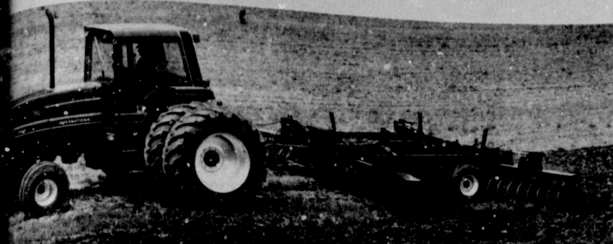
INTERNATIONAL HARVESTER 5288 tractor is one of the highest performance, high horsepower models in the 700 hp range. Its 6-cylinder, 466 cu. in. diesel engine develops 160 PTO hp. An all-new transmission provides 18 closely spaced forward and 6 reverse gears and combines the features of full synchronization and power shifting for efficiency and field performance. Like the other advance design models in the new series, the 5288 has a new drive train, forward air flow cooling, and Power Priority hydraulics, according to Brown's Implement, Ralls Highway.
