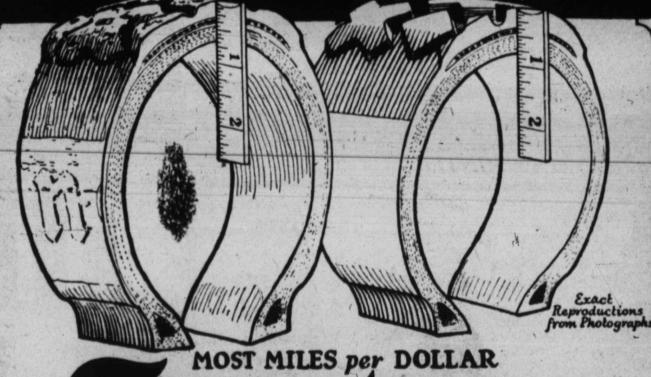
The tire section above at the left shows the condition of a Firestone 33x41/2 Cord Tire after 20,994 miles on a Yellow Cab in Chicago.
