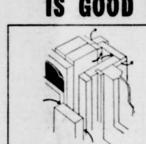
Arrows point to where cold air leaks in. TIGHT JOINT
