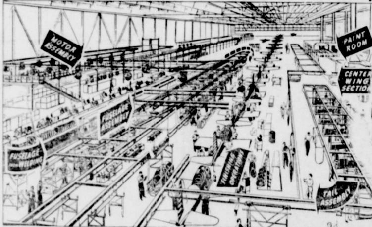
The above drawing of Vultee Aircraft's mechanized final assembly line shows the revolutionary production developments at the California plant in the last few months. It is the graphic story of how modern airplanes are made compared to the methods of but a year or two ago, and shows the first mechanized assembly line in the aircraft industry.
