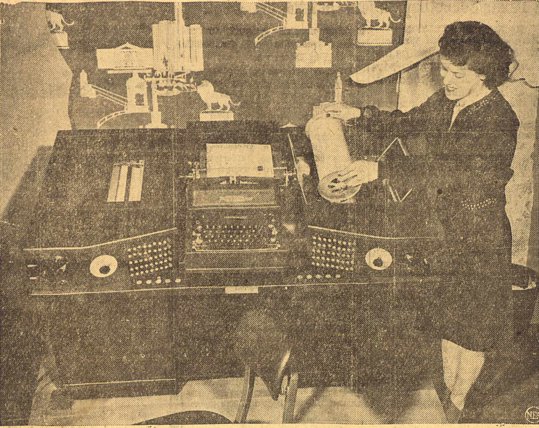
Push a button and this super typewriter writes a letter—almost. Displayed at recent Chicago office furniture show, it makes up business letters from numerous combinations of recorded paragraphs. Betty Lou Melchior is pictured installing recorded roll, similar to that used in player pianos. By pushing buttons, operator can pick paragraphs in the desired combination and machine types them.
