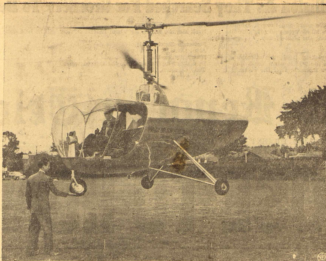
Stanley Hiller holds his new coaxial two-place "commuter" helicopter in the palm of his hand in a demonstration at Palo Alto, Calif.
