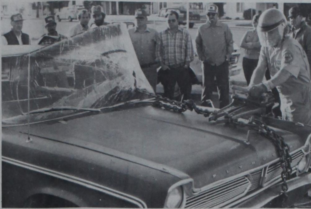
TONS OF FORCE —After first prying off the car's passenger door by outward force at the lock and the hinges, Gill reverses the jaw's mode to clamp-force, attaching the jaws to two chains, one of which is looped around the steering column and the other attached to the front frame. The result: the steering column
