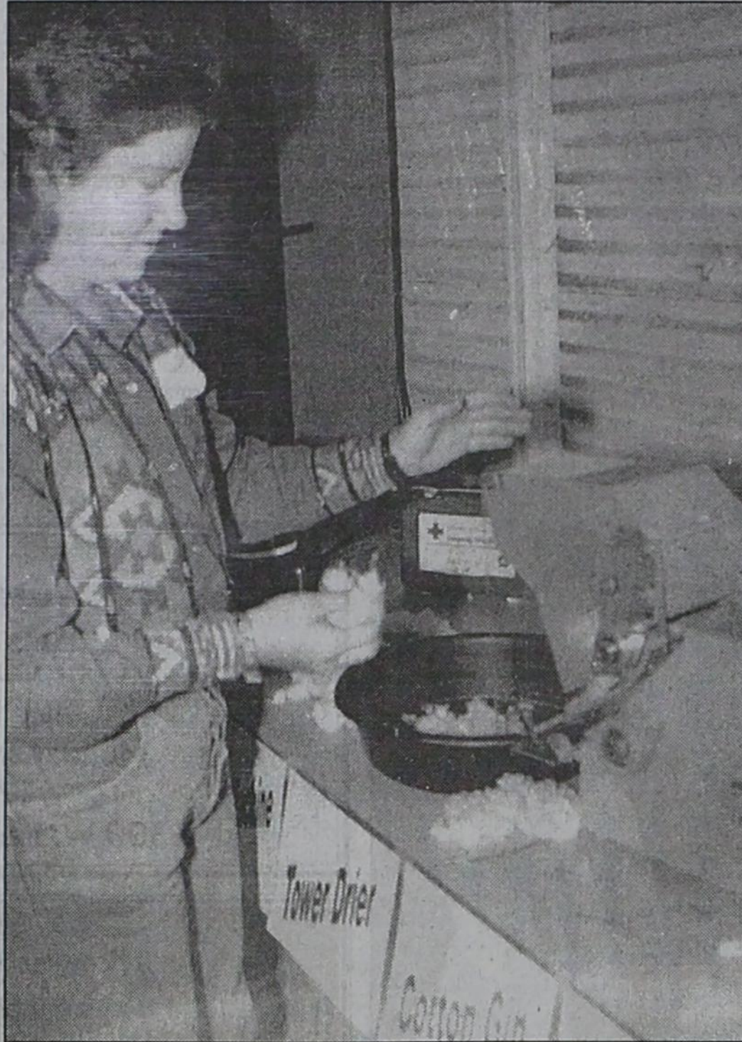
HERE'S HOW WE GIN COTTON —County Extension Agent Johnna Patterson feeds cotton into a machine and demonstrates how the seed and lint is separated during an exhibit at the Harvest Days celebration Saturday.
