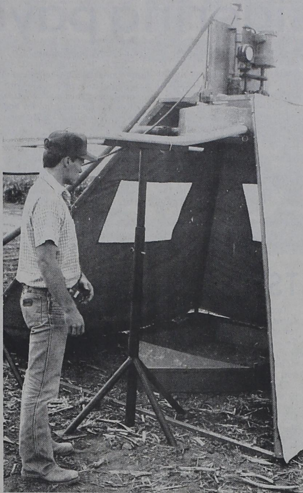
DAVID SWARINGEN of the High Plains Underground Water District demonstrates a "rainfall simulator" at the irrigation field day held Tuesday on the Danny Bruton farm south of Flagg. Swaringen's device can measure the effects of rainfall at rates from one-half to four inches per hour on a variety of soils and fields that are planted in a variety of methods and crops. The simulator can also help producers judge whether their fields are in need of nitrogen or other fertilizers.
