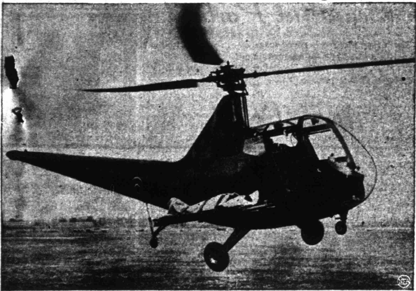
The Royal Air Force is testing a new method of evacuating casualties from battle areas. At this demonstration at Brize Norton, Oxford, England, a "wounded" soldier is strapped to the fuselage of the helicopter, which then takes off to rear air base. Special rigging is used to secure the litter to the plane.
