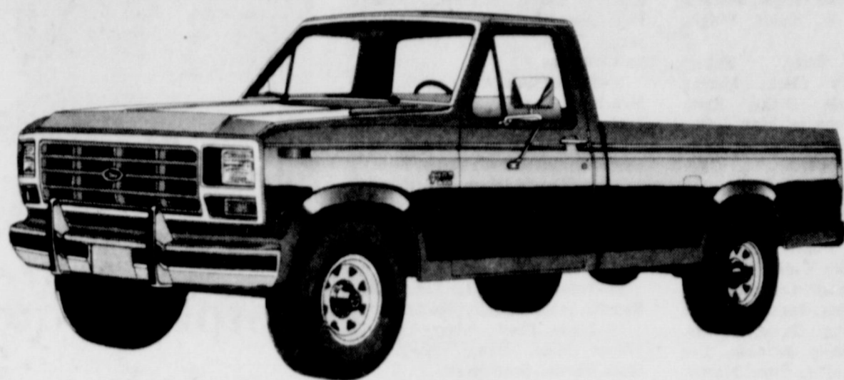
PU-3-82 F-100 XL STYLESIDE Options: Protection Group • Styled steel wheels (4) • Low-mount western mirrors • Rear contour bumper
