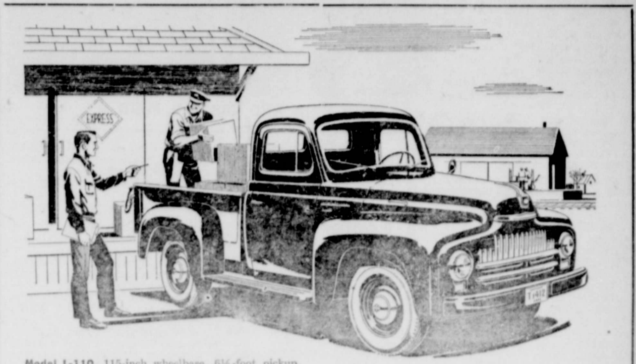
Model L-110, 115-inch wheelbase, 6 1/2-foot pickup body, 4,200 lbs. GVW. Pickups in the L-110, L-120 and L-130 Series include 115, 127 and 134-inch wheelbases, 6 1/2, 8 and 9-ft. bodies, GVW's to 8,000 lbs.
