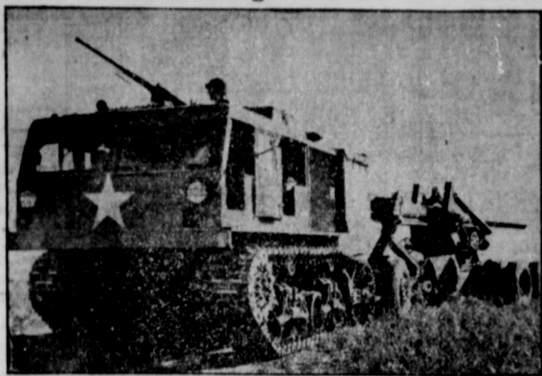
Soldiers at Fort Sill, Okla., Artillery Replacement Center find this new M4 high speed medium tractor a lot better than a truck. It carries a driver, 11 cannons, has space for 155-mm. gun ammunition, and can tow a "Long Tom" besides.
