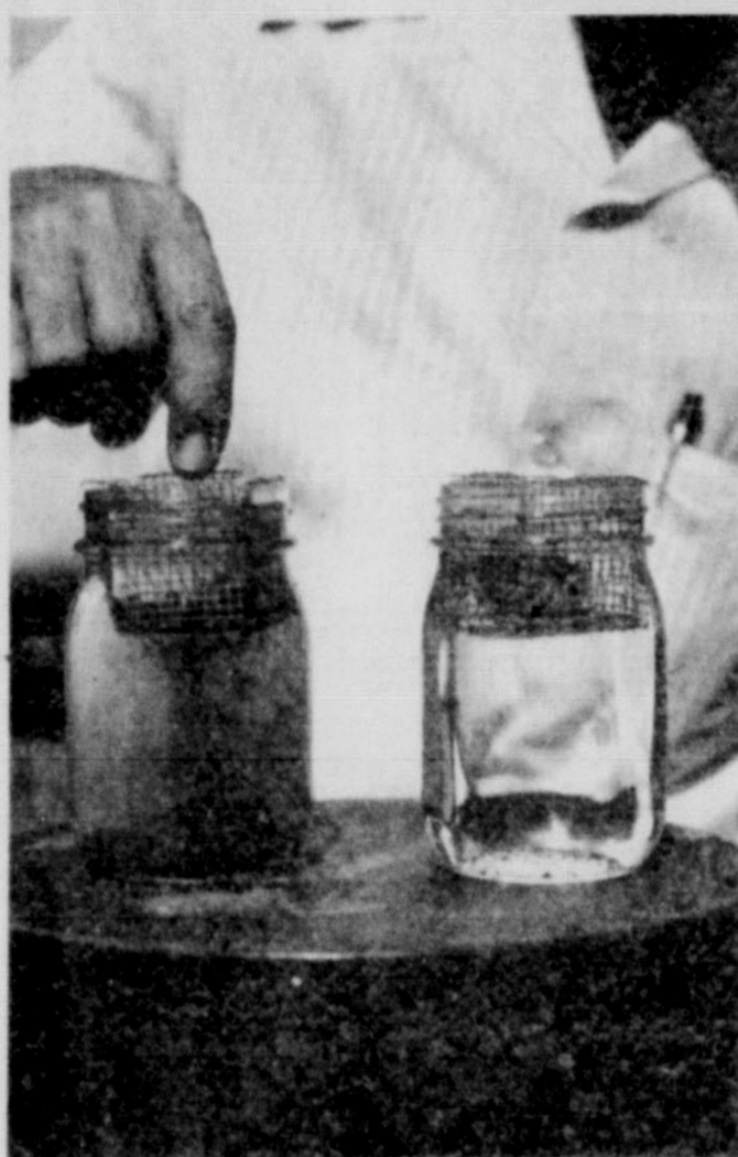
NO DOUBT ABOUT IT. The soil sample on the left is low in organic matter. For that reason, it breaks apart when immersed in the jar of water much more readily than does the sample on the right, which is high in organic matter. The sample in good condition absorbs water readily but does not break down and run together.
