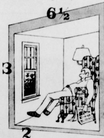
Insulation should be at least 6 1/2 inches thick in the ceiling, 3 inches thick in walls and 2 inches in floors.
