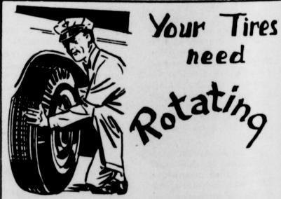
Front tires are subject to wear from steering and braking. Rear tires are worn by the forces of driving, stopping and holding on curves. To equalize this wear and increase tire mileage, tires should be rotated regularly so that they will run in different positions.
