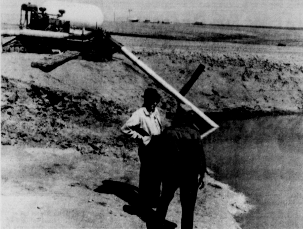
ONE OF THE COUNTY'S many lake pumps in the area which makes use of tailwater is this one located on the Gilbert Wenner farm south of Friona. Wenner's pump has been gauged at 72,000 gallons per hour. Allan White and Wayne Wyatt of the High Plains Underground Water Conservation District are seen in the foreground.
