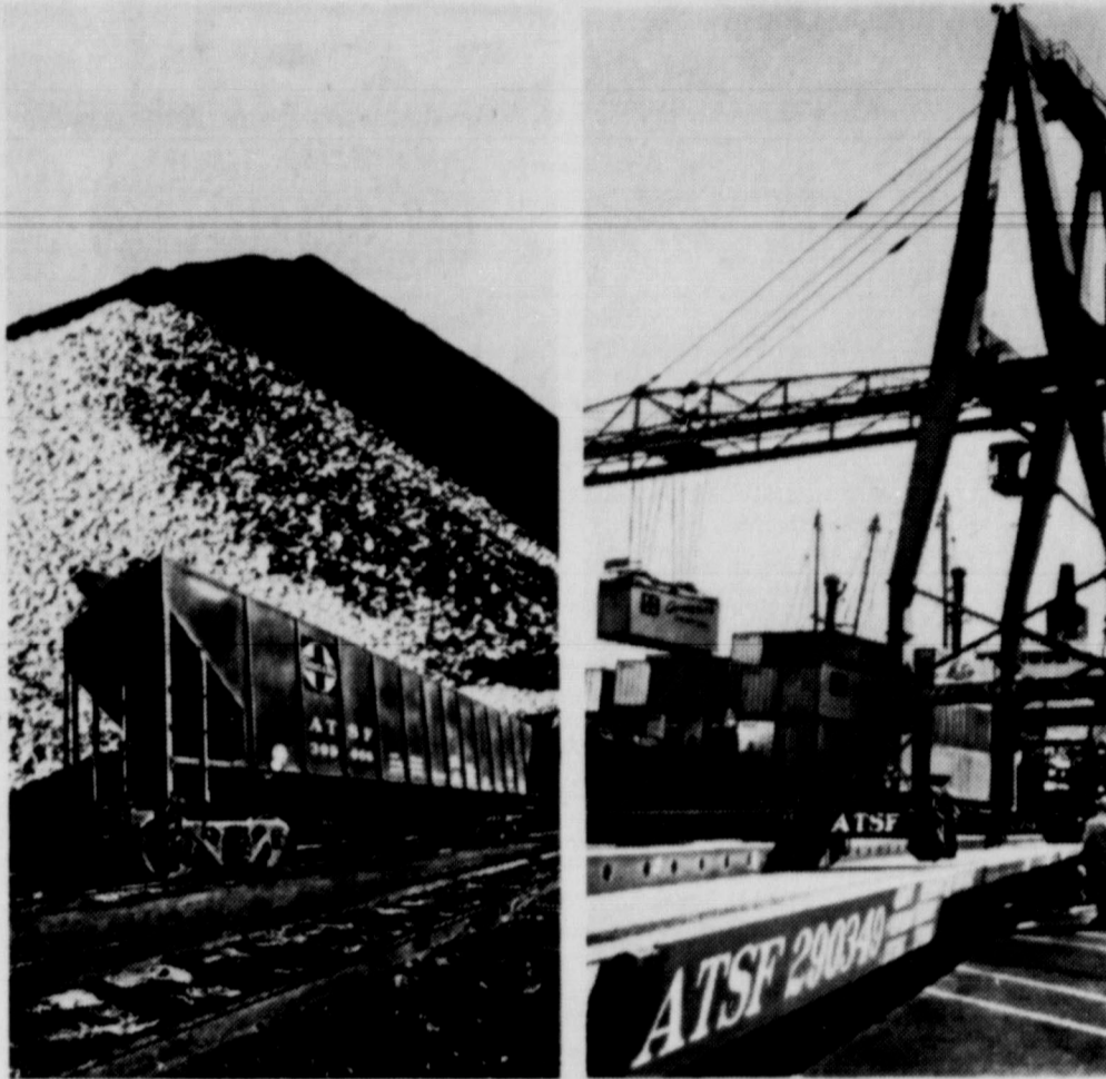
Santa Fe has more than 8,750 huge 100-ton covered hopper cars (left photo). Each one can be loaded or unloaded in minutes, providing a fast, economical way to move mountains of bulk commodities such as grain, potash, cement, to market or manufacturing plant.
