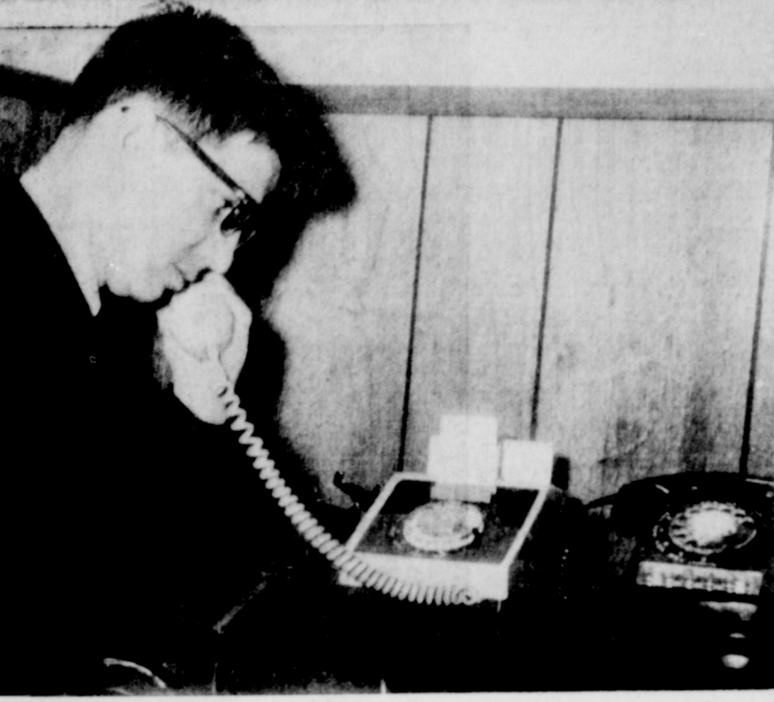
The new beside the old . . . MORTON AREA Chamber of Commerce Manager John Johnson is shown using a self-dialing telephone believed to be the first of its kind in this area. The new telephone uses a punch-card system to dial numbers automatically. TRIBpix.
