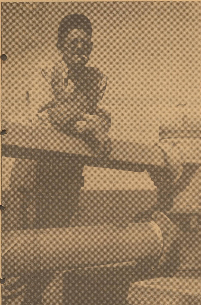
MAKING THE WELLS SAFE —At the left, A. G. "Gus" Schlab of Black leans on a power shield to demonstrate how well it protects the moving parts of the drive shaft from his irrigation well engine to the gearhead. At right,
