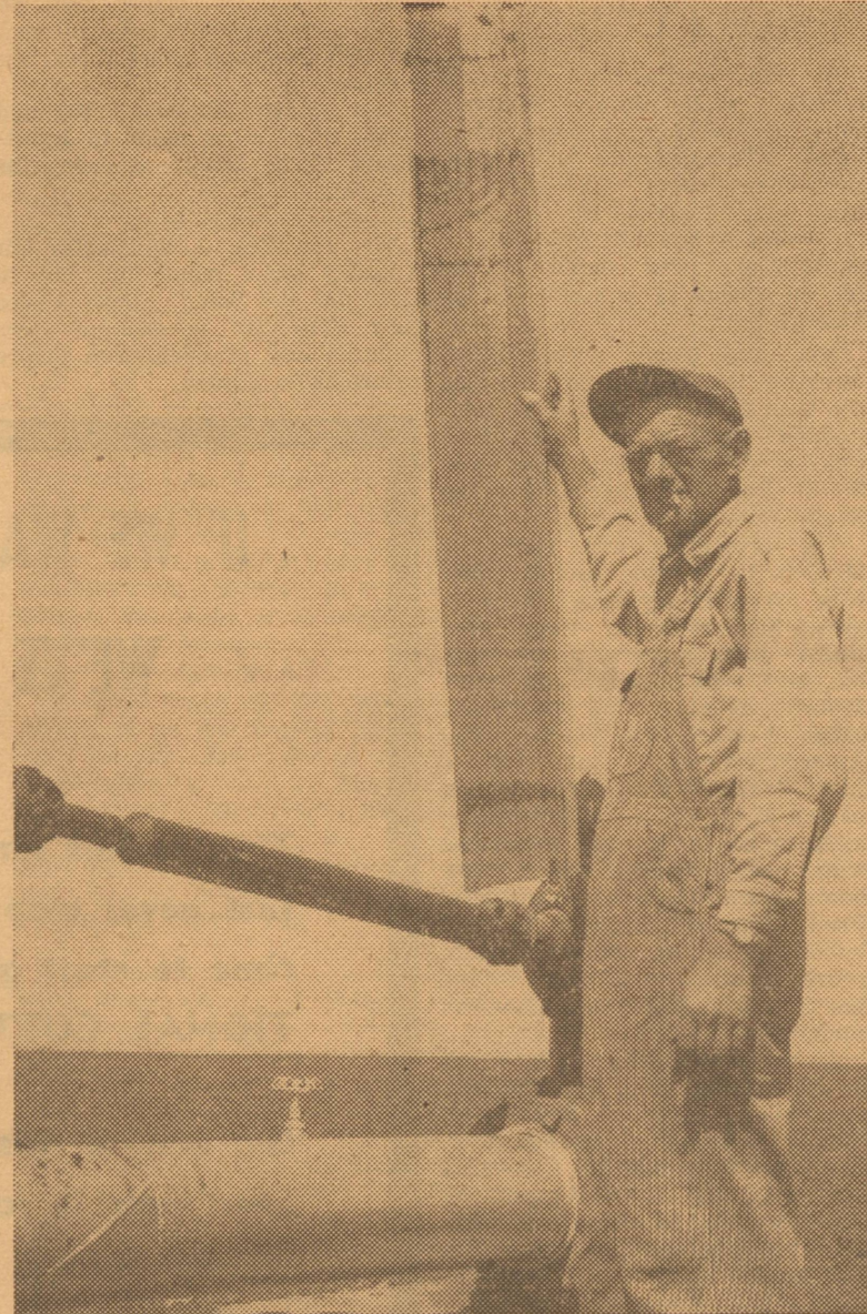
he lifts the shield, which is hinged, to demonstrate how easily the moving parts are made accessible for greasing or other maintenance.
