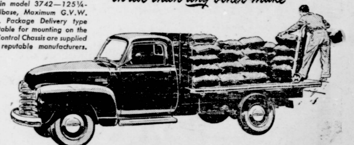
MEDIUM-DUTY CAB AND CHASSIS WITH PLATFORM BODY Model 3808—137-inch wheelbase, Maximum G.V.W. 8,800 lb. Other models available up to 161-inch wheelbase and 16,000 lb. G.V.W.
