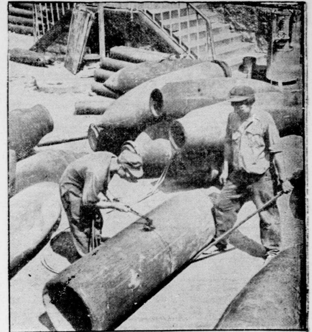
LEFT OVER FROM THE BLITZ—Workmen in Berlin use an acetylene torch to carve up a two-and-a-half-ton block of scrap iron. Originally destined for England via the Luftwafer, the bombs are among hundreds of tons of scrap iron and steel being shipped daily to England by a more peaceful water route.
