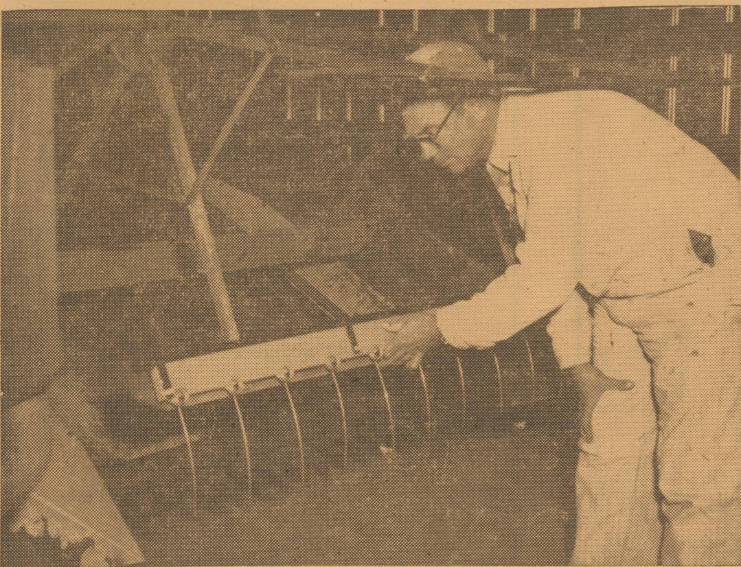
These steel tines or fingers enable R. L. Douglas, Bovina area farmer, to harvest soybeans with improved efficiency. He is equipping a small combine with special attachments to permit him to get the most from his 'bean crop this year.
