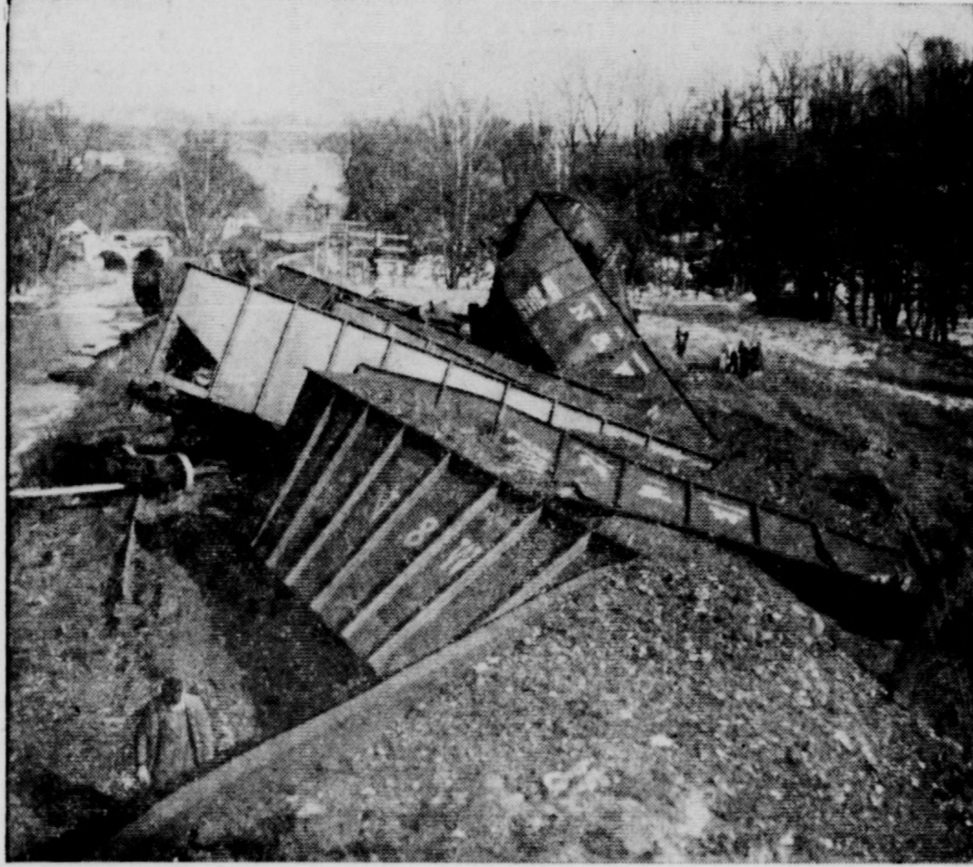
TEMPORARILY OUT OF SERVICE —A broken rail resulted in the wreckage of 16 loaded coal cars near Wheeling, W. Va., and rail service was disrupted for 12 hours. The rest of the 45-car train remained on the tracks as wrecking crews struggled to clear and repair the damage.
